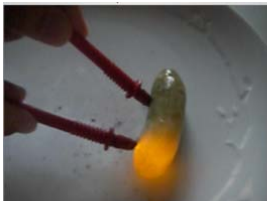
Figure 1 Arcing inside the pickle causes it to glow. Arcing can occur at either electrode.
