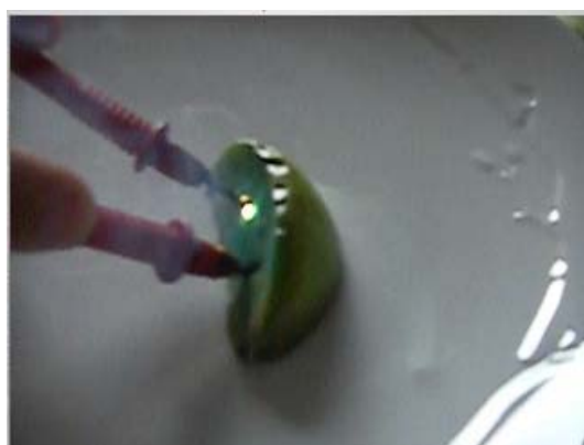
Figure 3 Apple soaked in copper sulfate produced weak arcing with low intensity light. The light had a slight greenish tinge
