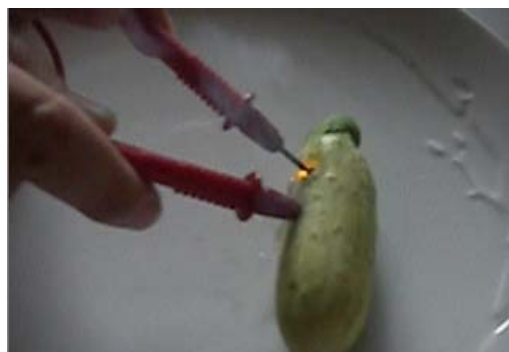
Figure 2 Electrodes must be closer together for arcing to occur in raw vegetables and the light intensity was significantly lower.
