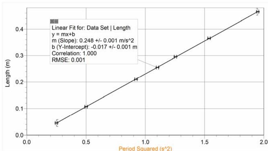
**Fig 9:** Length of mean water column versus Period Squared for small amplitude oscillations. The relationship is linear within uncertainty, showing that the oscillation is simple harmonic motion and the end correction is independent of column length, as predicted by equation 6.
