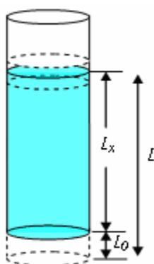
**Fig 4:** Water Tube and End Correction
