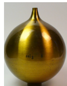
Figure 1 A classic Helmholtz resonator. 1
