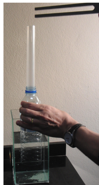
Figure 2 The water bottle with extended neck and bottom cut off was adjusted to find the position of maximum resonance.
