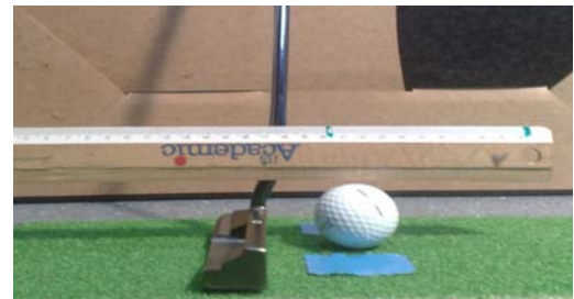
Figure 1 The experimental set-up. A putter in putting position with the ball and a ruler as reference frame directly over the ball.
