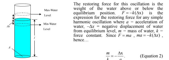
Fig 3: Water oscillation in a tube
